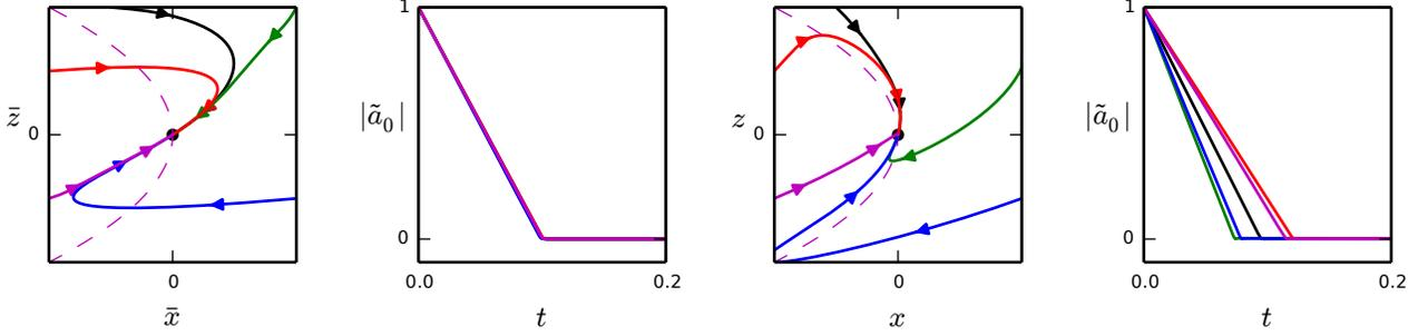
Fig. 1. Left: trajectories of the closed-loop system (15) under the nonlinear adaptive controller of Proposition 1. Right: the error norm  $|\tilde{a}_0| = |a_0 - \hat{a}_0|$  of the trajectories plotted on the left. For these plots we have used parameters  $(a_0, a_1, a_2, r, c_0, c_1, d_0, \gamma_0) = (1, 2, 3, 0.5, 1, 7, 100, 0.1)$ , and initial condition  $\hat{a}_0(0) = 0$ .
