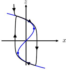
Fig. 3. Open-loop phase portrait of the van der Pol oscillator (28). The (blue) S-shaped manifold represents the critical manifold  $S$  defined by (29). The system has two fold (jump) points located at  $\pm (\frac{2}{3}, 1)$ .
